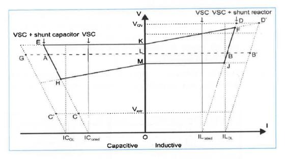
Figure-3: VI Curve of the STATCOM Station
