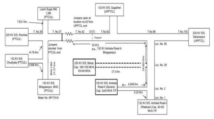
SINGLE LINE DIAGRAM OF THE LILO OF 132 KV SAHARANPUR-BHAGWANPUR/ROORKEE LINE
