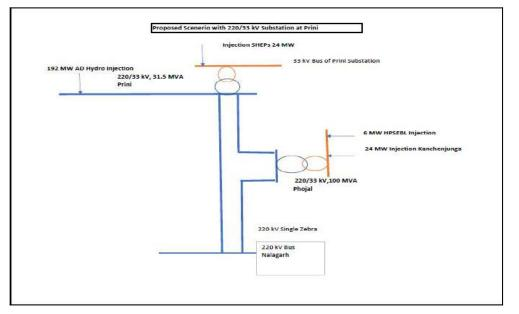
Accordingly, HPPTCL has proposed the construction of Prini 220/33 kV, 31.5 MVA substation by HPPTCL in AD Hydro Switchyard at Prini alongwith one number of 220kV bay at Prini.
